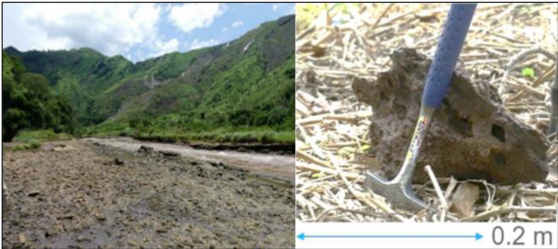
Figure 7-21 River Bed Alluvium at the Project Dam Site Cemented Alluvium Exposed on the Bed at the Dam Site (left) and a closeup of a portion of the calcrete layer (right) (Source: Tractebel, 2021a).
